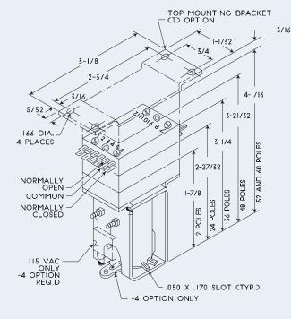
52 POLES USES ONLY POLES NOS. 1, 6, 7 AND 12 ON TOP DECK .100 X .060 SLOT (TYP.) .100 X .060 SLOT (TYP.) .100 A .060 SLOT (TYP.) .12 34 5 6 .12 34 5 6
